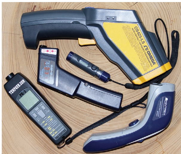
Fig. 1. The five models of IR thermometers used in the precipitable water vapor study.
